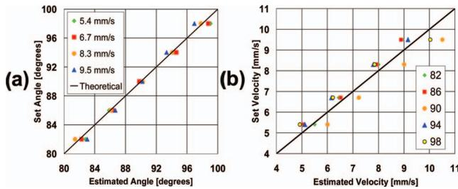
Fig. 2. Estimation of (a) Doppler angle and (b) velocity using the dual-angle, delay encoded technique. Solid line, unity slope.
